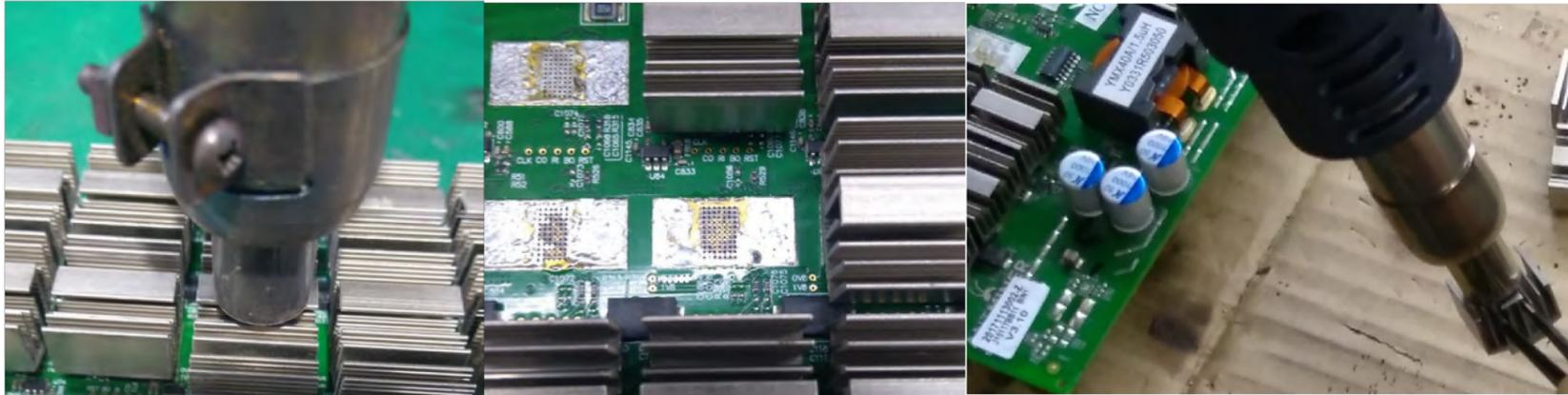
**Disassemble the cooling fin on the back, heat the cooling fin on the back until the temperature is high enough to melt tin, and then use tweezers to remove it. In assembly, heat outside first until the temperature is high enough to melt tin, place the cooling fin on the pad and press.**
