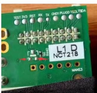
Add an IUF 0603 capacitor between pin 1 and pin 2 of O2 on the back of IO Mouth
