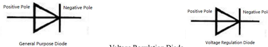
The symbols of diode in circuit
