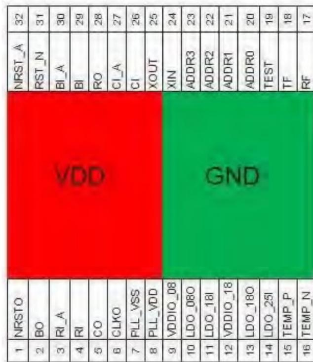
Fig 6. BM1387 Chip Pins
